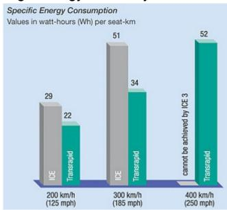
Transrapid energy efficiency compared to German ICE conventional steel-wheel fast trains.
