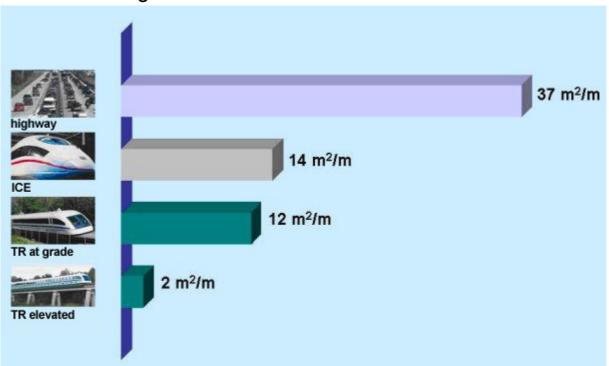
Transrapid system land use compared to motorways and German ICE conventional steel-wheel fast trains.
