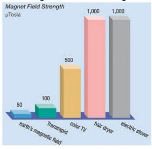
Transrapid magnetic field strength inside the cabin compared to a hair dryer and other domestic appliances.
