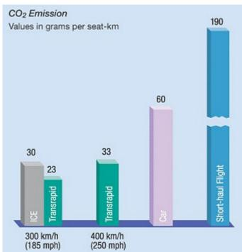
$\label{eq:conventional} \textbf{Transrapid CO}_2 \ \textbf{emissions compared to German ICE conventional steel-wheel fast trains, cars and aircraft. } \\$
